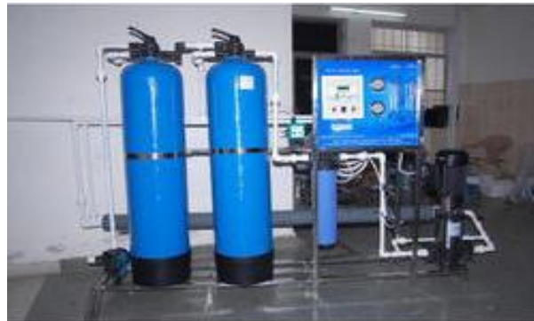
500LPH RO IN FRP PENTAIR HOUSING.
